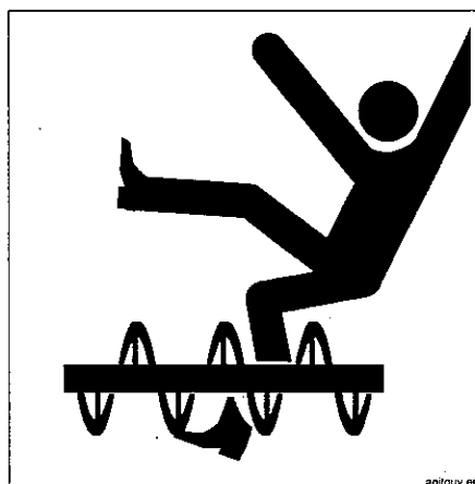
Figure 2 - addendum Lifting hopper grate exposes the agitator and the concrete valve
